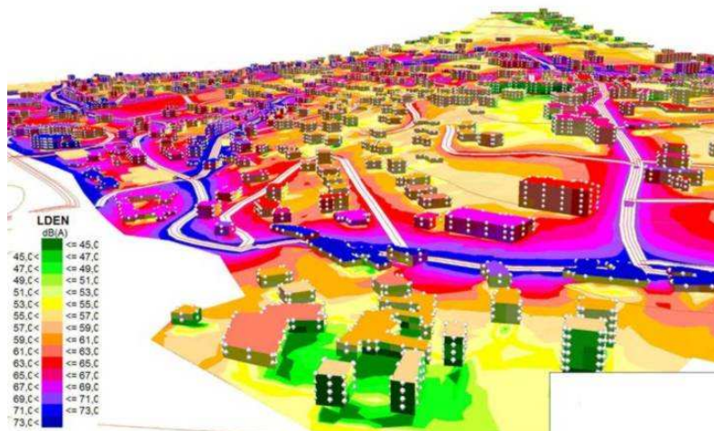
Above: 3D graphic representation of the level noises measured prior to the works
