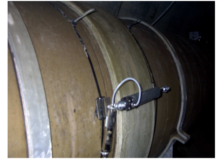
Above (From left to right): View down the tunnel showing the location of one of the CCTV LED cameras. Geophones mounted on the pre-cast concrete lining and the GRP pipes. High precision crack gauge (accurate to 0.1mm) installed over one of the GRP pipe joints.
