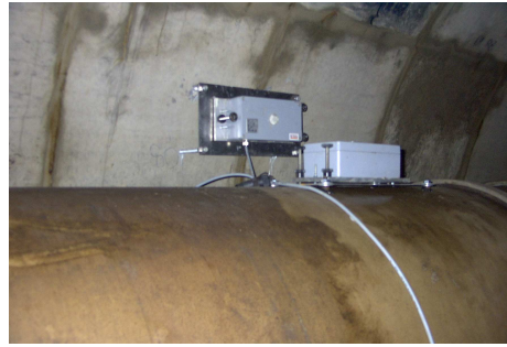
Above (From left to right): View down the tunnel showing the location of one of the CCTV LED cameras. Geophones mounted on the pre-cast concrete lining and the GRP pipes. High precision crack gauge (accurate to 0.1mm) installed over one of the GRP pipe joints.
