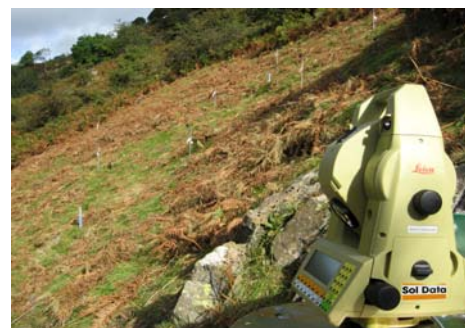
Cyclops providing real time slope displacements to the client
